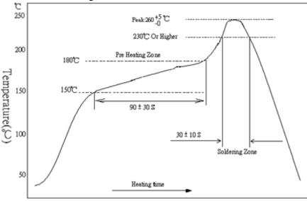
Remark: The peak temperature of soldering heat is 260 +5/-0  $\,^\circ\!\mathrm{C}\,$  for 10 seconds.
